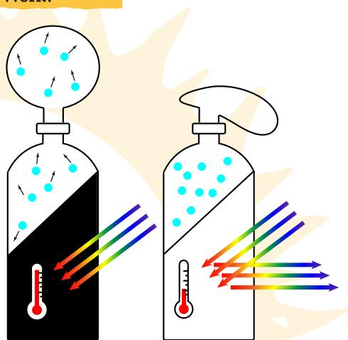
This experiment works by taking advantage of how different colors absorb or reflect different wavelengths of light. Pigments like the ones in the paint you used to cover your plastic bottles work by absorbing certain wavelengths and reflecting others. For example, if you are wearing a blue shirt the blue pigment in your shirt's fabric is absorbing every wavelength but blue, reflecting blue back to the eye as you look at it.
